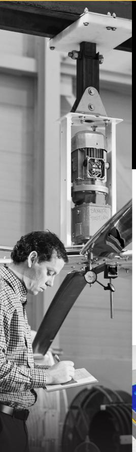
HVLS fans utilize efficient, relatively small horsepower drive units along with large airfoils to deliver big airflow over a very large area – at a modest and safe RPM. Thanks to their precise aerodynamic design, Big Ass Fans efficiently move massive air volumes and dramatically improve comfort even in harsh environments.
