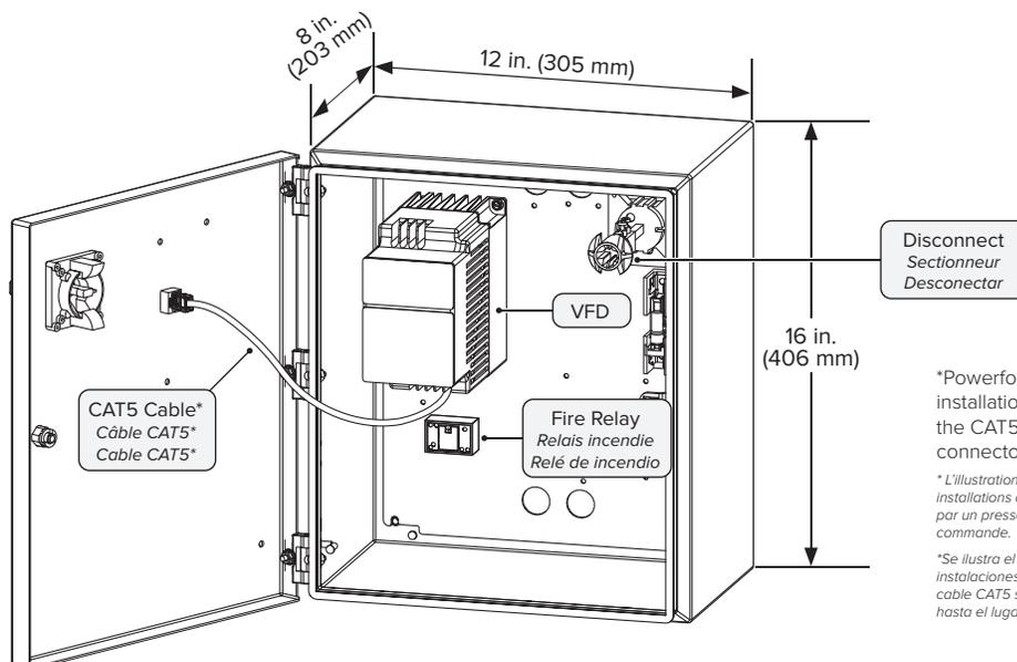
\*Powerfoil X3.0 Washdown enclosure shown. For installations with a remotely-mounted wall controller, the CAT5 cable is routed through a conduit connector to the controller installation location.
