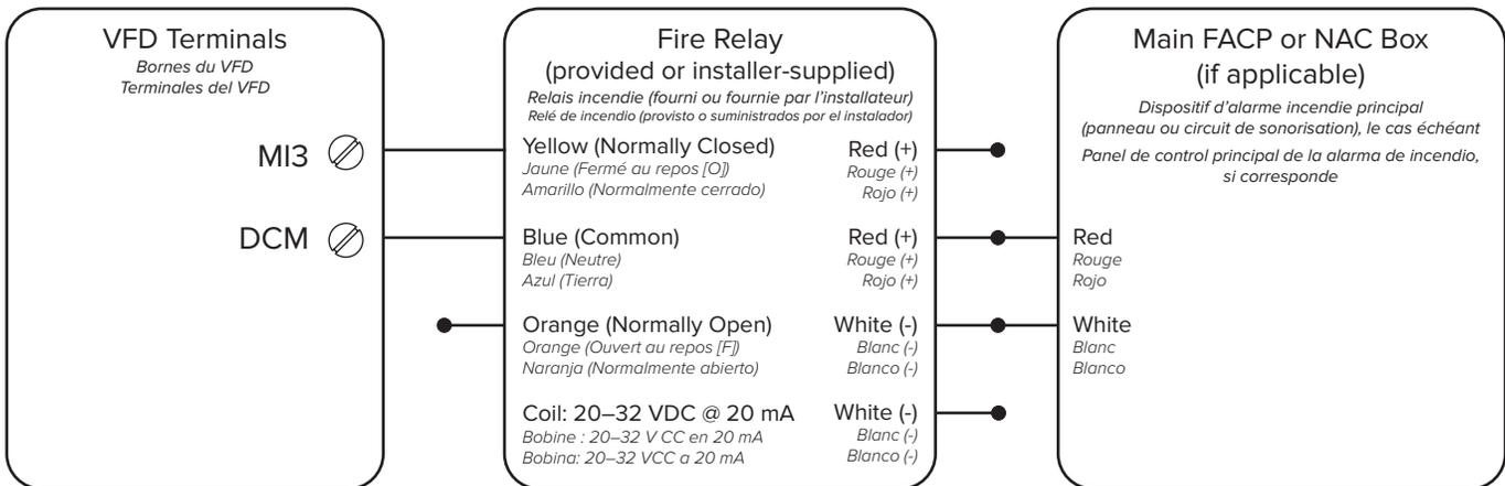
The relay coil must remain energized with 24 VDC by the FACP for fan operation. This would be considered a fail safe or fail open wiring arrangement. This is done using one set of the red (+) and white (-) wires. The other set of red and white wires is for passing the signal to the next fan (supervised pass-through). An alarm condition will stop the fan and issue a fault at the controller.
