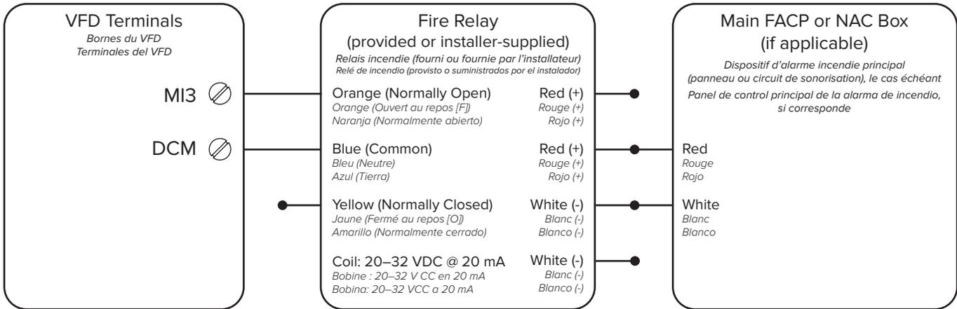
A contact closure across digital input terminals MI3 and DCM will result in fan shutdown. The relay coil must be energized with 24 VDC by the FACP for fan shutdown. This is done using one set of the red (+) and white (-) wires. The other set of red and white wires is for passing the signal to the next fan (supervised pass-through). An alarm condition will stop the fan and issue a fault at the controller.
